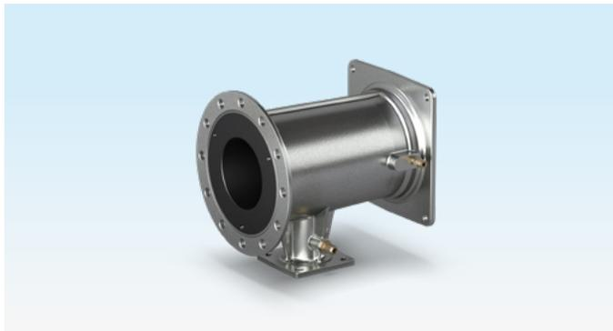
The venturi mixing unit allows modulation of a premix burner with a constant gas/air ratio down to 14 to 17% of maximum load.
