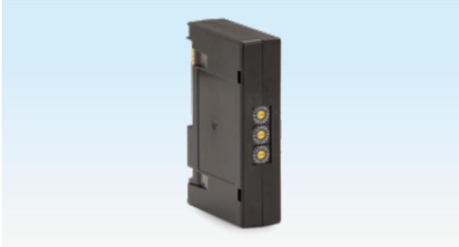
The bus module BCM 400 is used as a communication interface for devices of the BCU 4 (2019) product family for connection to a fieldbus communications system (PROFIBUS, PROFINET or EtherNet/IP). Networking via the fieldbus enables the BCU to be controlled and monitored by an automation system (e.g. PLC).
