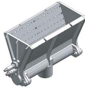
MAXON Series "NP" & "RG" AIRFLO® burners consist of a robust cast-iron or aluminum burner-body (which serve as the gas manifold) drilled to discharge the gaseous fuel between diverging stainless steel mixing plates.
