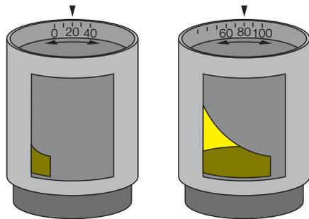
Fig. 7: Flow restricting cylinder and linear slide control valve for linear flow control LFC
