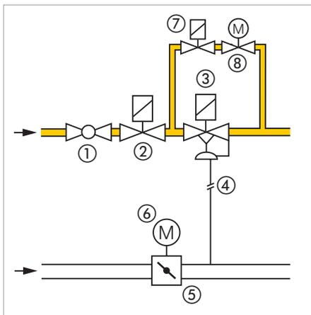
**Fig. 3:** Modulating air/gas ratio control with bypass line for cascade control
