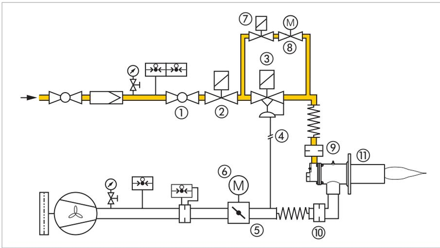
Fig. 6: Heating installation as per EN 746, Part 2
