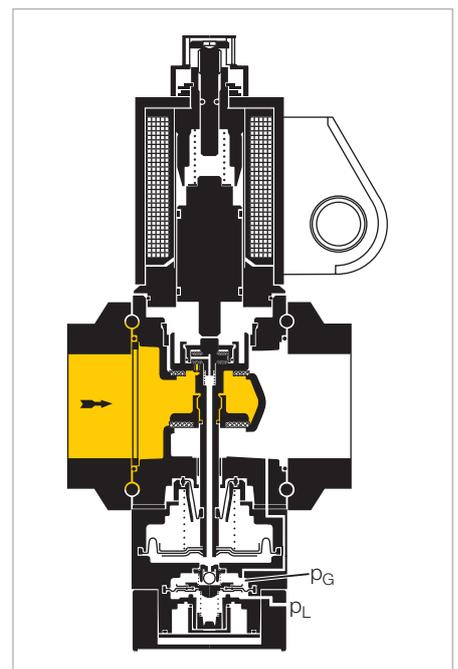
Fig. 2: Section of Type VAG air/gas ratio control with solenoid valve
