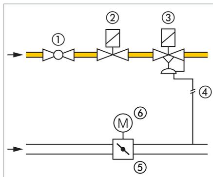
Fig. 1: Modulating air/gas ratio control – standard version
